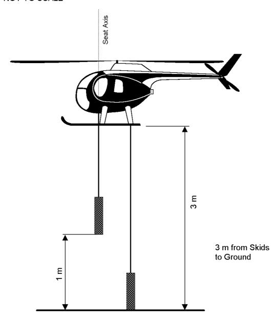
It is essential to unterstand that from one helicopter to another, the short rope will differ in size. The objective is to have 1 metre difference between the bottom of the two weights.
