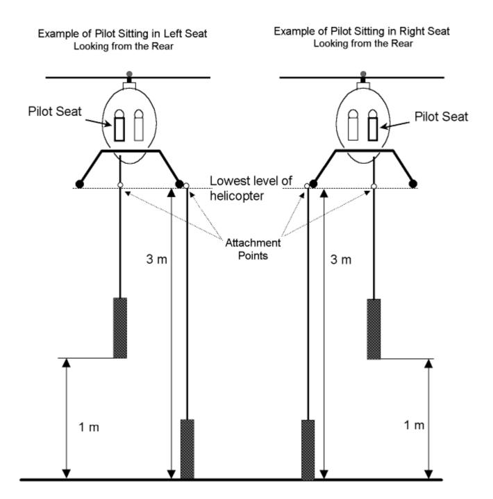
The long rope will always be on the opposite side of the helicopter to the pilot. Attachement on skid or wheel.
