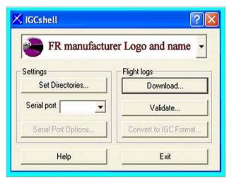
Method - Stage 1: Make sure that the manufacturer's DLL file for your type of FR is in the same directory as the IGC Shell program. On executing the IGCshell.exe file you should see the screen shown in the picture. Select the appropriate FR manufacturer and FR name by scrolling though the list in the top box of the screen. Then select the function required (Validate, Download etc).
