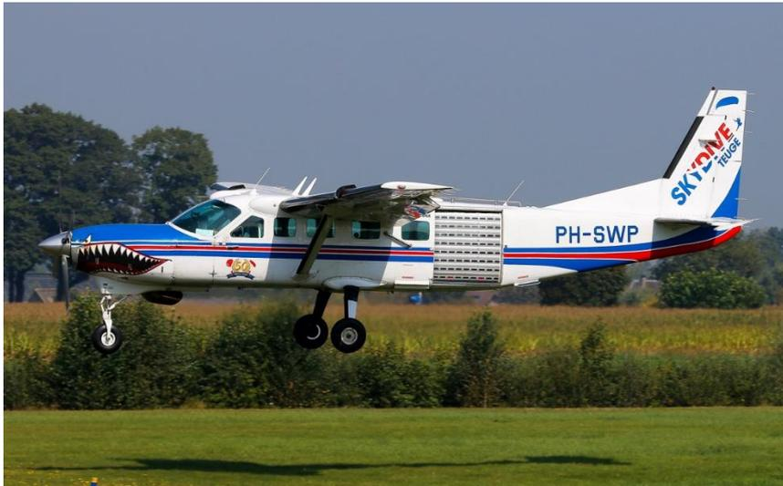
3X Cessna 208B Supercub are available for all events. All aircraft have one engine (900 shp), can seat a maximum of 18 skydivers with a left-hand door, all with the same dimensions. All aircraft have both rear and front video step with handles on the outside and inside.
